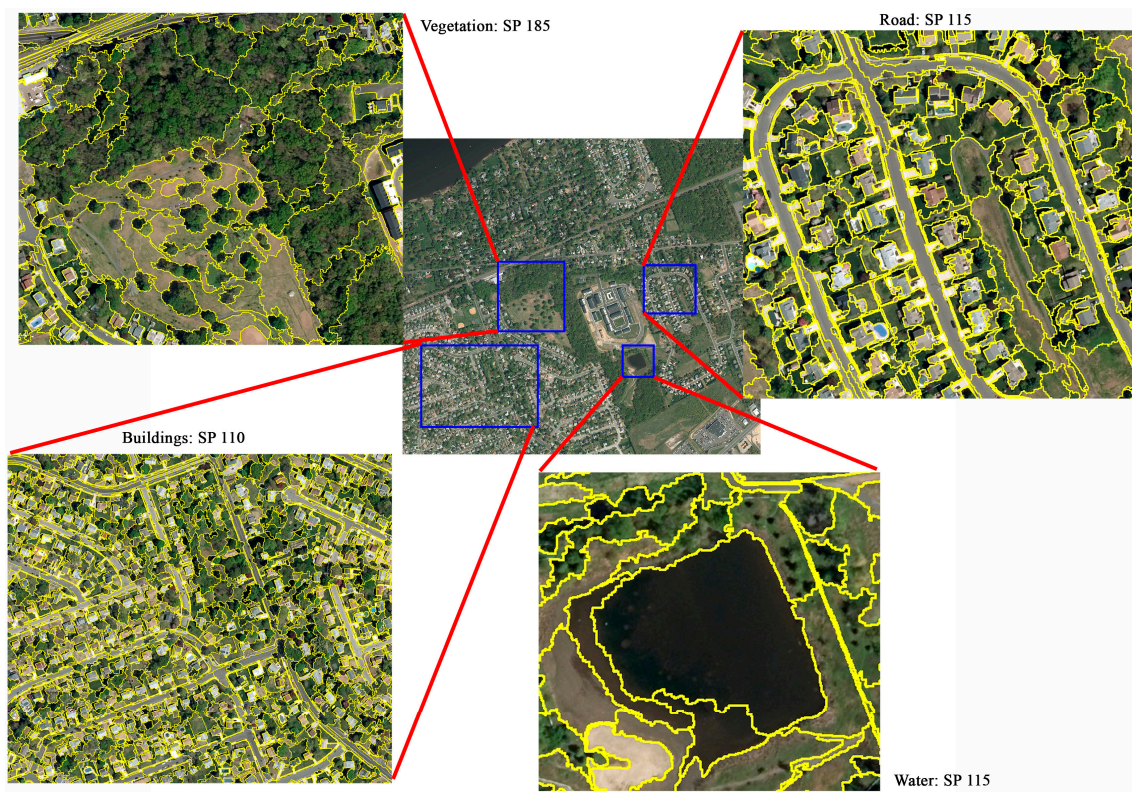
Figure 4. Segmentation results of the building, vegetation, road, and water classes in the 30-cm test image.
