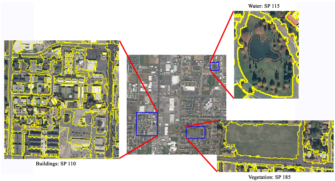
Figure A1. Segmentation results of the building, vegetation, and water classes in the 25-cm test image.
